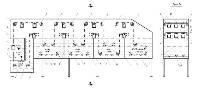
**Fig. 1.** Device for multilevel high-temperature thermal sterilization of fruit and vegetable canned goods in liquid high-temperature heat carriers using secondary heat resources. It contains a frame 1, heating elements 2, sprockets 3, separators 4, baths for heating and cooling 5 and 18, Gall's chain 6, bath for cooling 7; showers 8 and 12, inbound transporter for cans 9, outbound transporter for cans 10, can carriers 11, a drive sprocket 13, shafts 14, guides 15, bearings 16, and corners 17.
