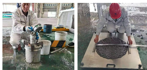
(a) Air content test (b) Slump flow test and T500 test
