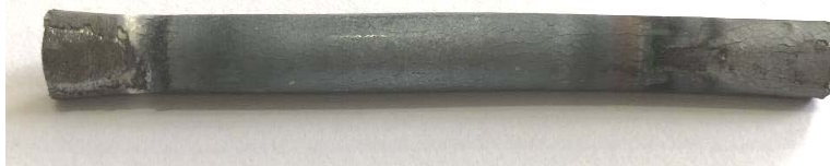
Fig. 12. Thermal-cycle test sample after 1050 times ranging from 1700°C to room temperature.
