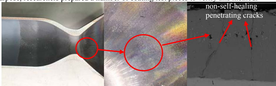
Fig. 10. A big number of non-self-healing penetrating cracks were formed in the large temperature gradient region at downstream of the throat.
