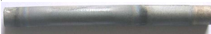
Fig. 11. Static high-temperature test sample after 30h at 1800°C.
