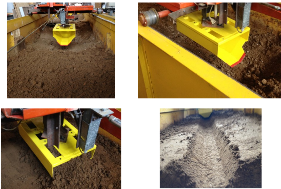
Fig. 3. Testing the working body model of a canal cleaner in laboratory conditions
