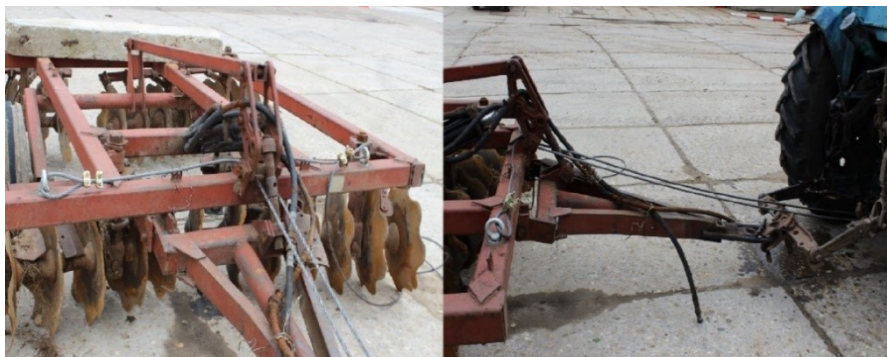
Fig. 2. General view of a tractor with a harrow unit coupling weight regulator
