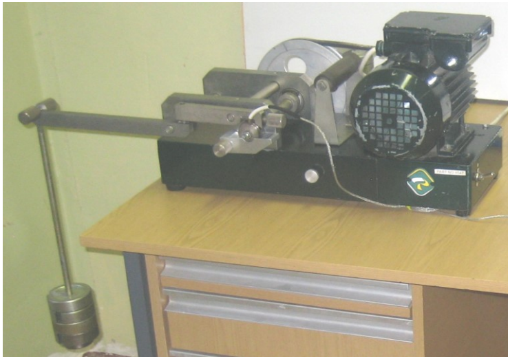
Fig. 2. General view of the modernized Timken-Machine
