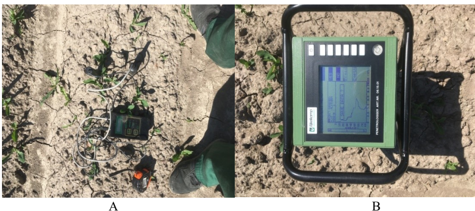
Fig. 2. Soil moisture meter manufactured by "TR di Turuni & c.Snc" (a), penetration logger from Eijkelkamp (b)
