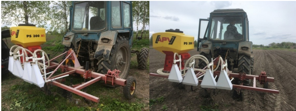
Fig. 1. Multipurpose row-crop cultivator for inter-row cultivation of potato plantings with deep loosening of row spacings and simultaneous sowing of cover crops
