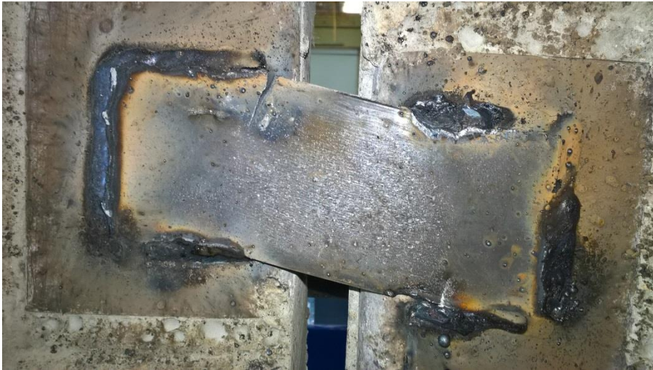
Fig. 5. Destruction of the connecting plate welded butt.
