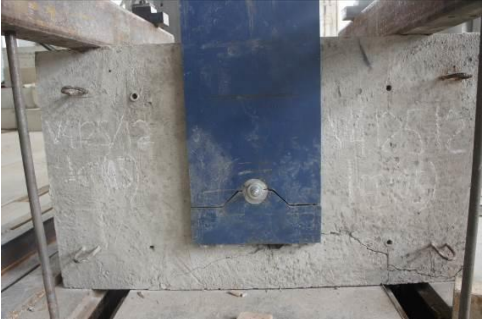
Fig. 3. Rig for anchor shear tests.
