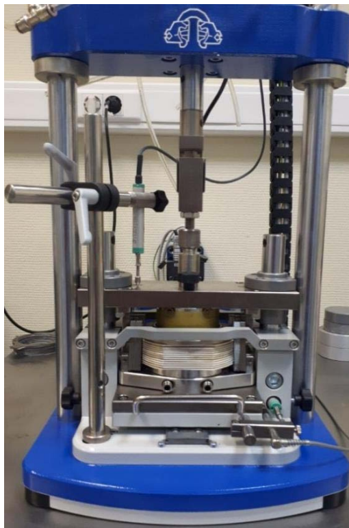
Figure 1. Simple shear device manufactured by «NPP Geotek».
