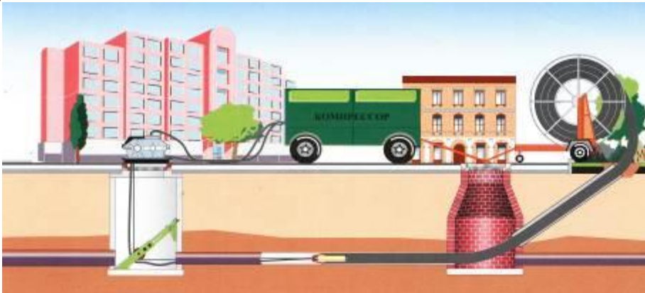
Fig. 5. Rehabilitation of a section of a worn water distribution network without destruction by pulling polymer pipes.
