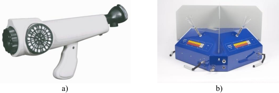
Fig. 1. Mobile olfactometer (a) and laboratory olfactometer (b).
