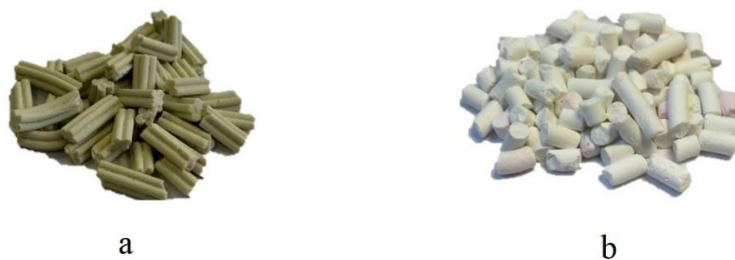
Fig. 3. Catalyst support forms of extrudates: a – modern catalysts, b- domestic catalysts.
