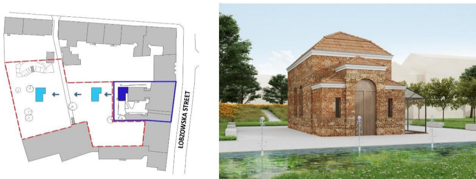
Fig. 3. On the left - schematic diagram of the two possible new locations of the building: the current place of the Atelier and a plot with tenement house marked in dark blue, possible locations marked in light blue; on the right – visualization of the regeneration project made by the author.
