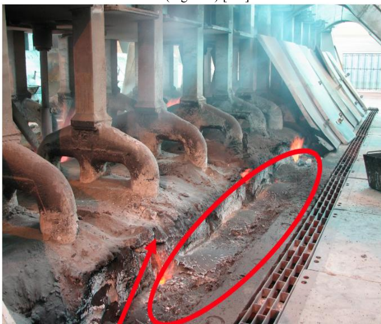
Fig. 1. The crust of cryolite melt.
