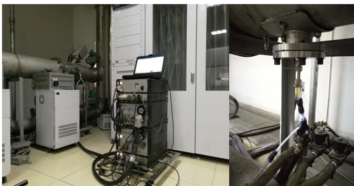
Fig. 2. Connection mode of PEMS and CPC 2000 sampling probe.
