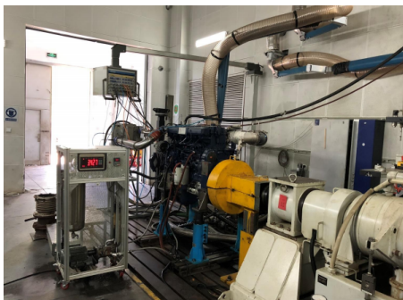
Fig .1. Engine bench and main test equipment.
