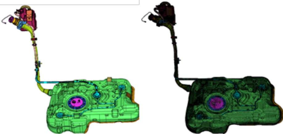
Fig. 1 (a) 3D model of fuel system.
