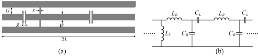
Fig. 1. The proposed supercell CRLH leaky-wave structures. (a) Layout. (b) Equivalent circuit model.
