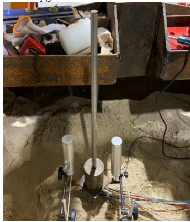
(a) Pile top impact test device
