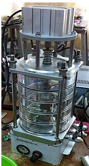
Fig. 1. Triaxial compression device – stabilometer.
