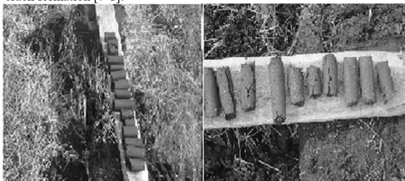
Fig. 3. Molded peat pieces: on the left - immediately after molding; on the right - after 20 hours of drying under conditions of polar day.
