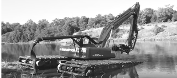
Fig.1. Swampking Pontoon Excavator with Powerful Dredger PD 3000.
