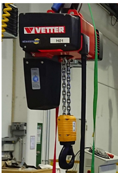
Fig. 3. Chain hoist with 2/1 reeving system.
