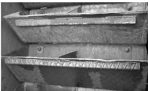
Fig. 3. Elevator buckets made of corrugated flooring at Pindstrup LLC.
