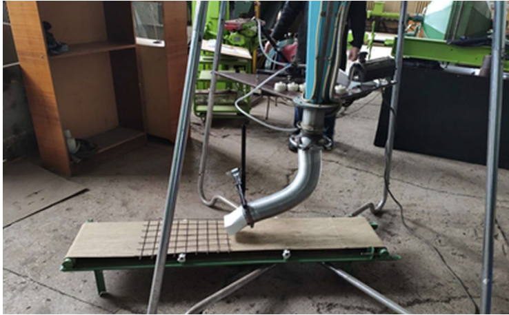
Fig. 4. Coordinate grid on the conveyor belt.
