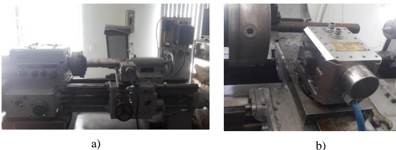
Fig. 1. Experimental equipment, a) machine 1k625, b) measuring stand STD. 201-1
