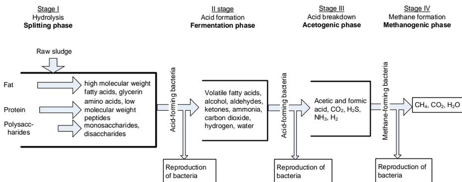
**Fig. 1.** Schematic diagram of biogas synthesis.
