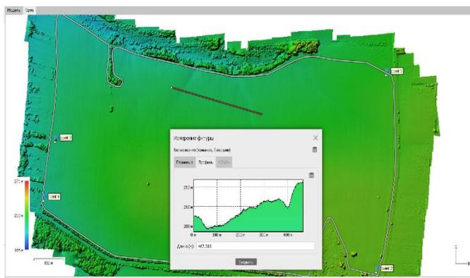
**Fig. 11.** DTM with a constructed profile along the givenline, maximum slope 4% (2.29 degrees).
