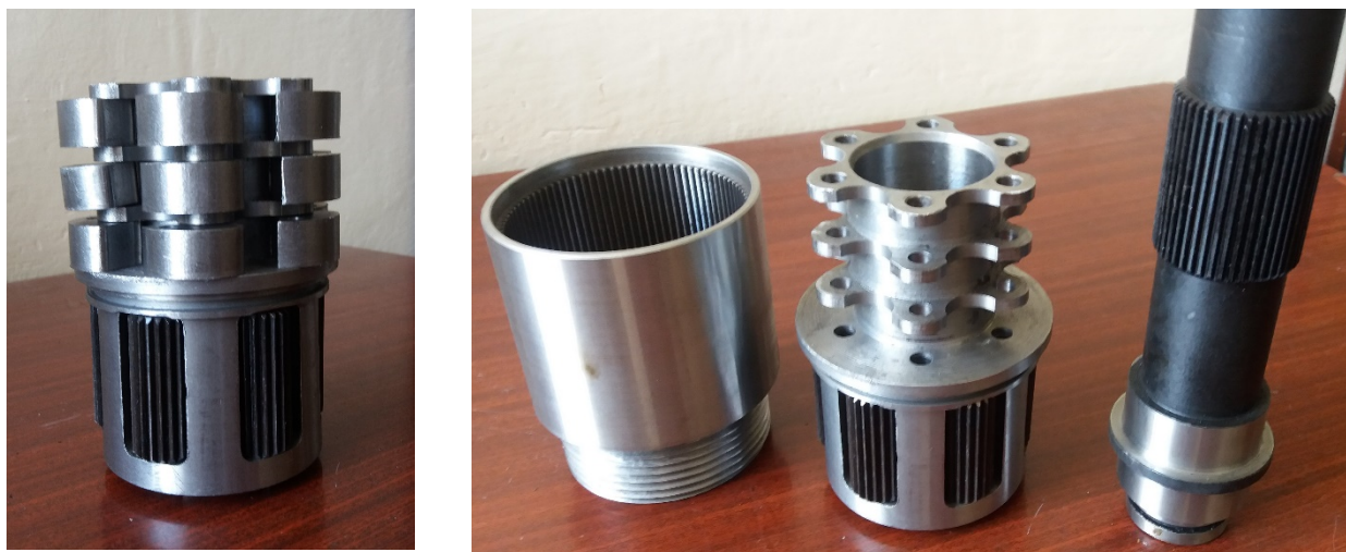
Fig. 3. Laboratory experimental model of a device for unscrewing a captured column of pipes.
