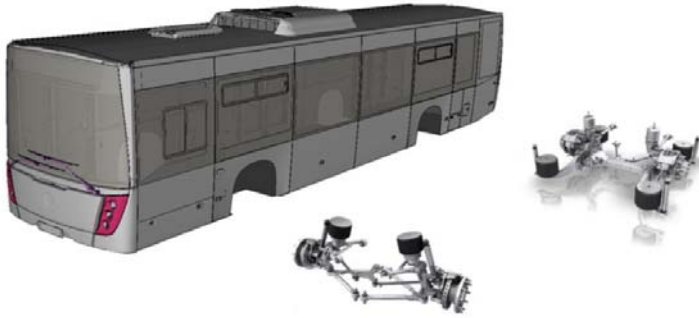
Fig. 4. Virtual bench for assessing acoustic noise inside a vehicle.
