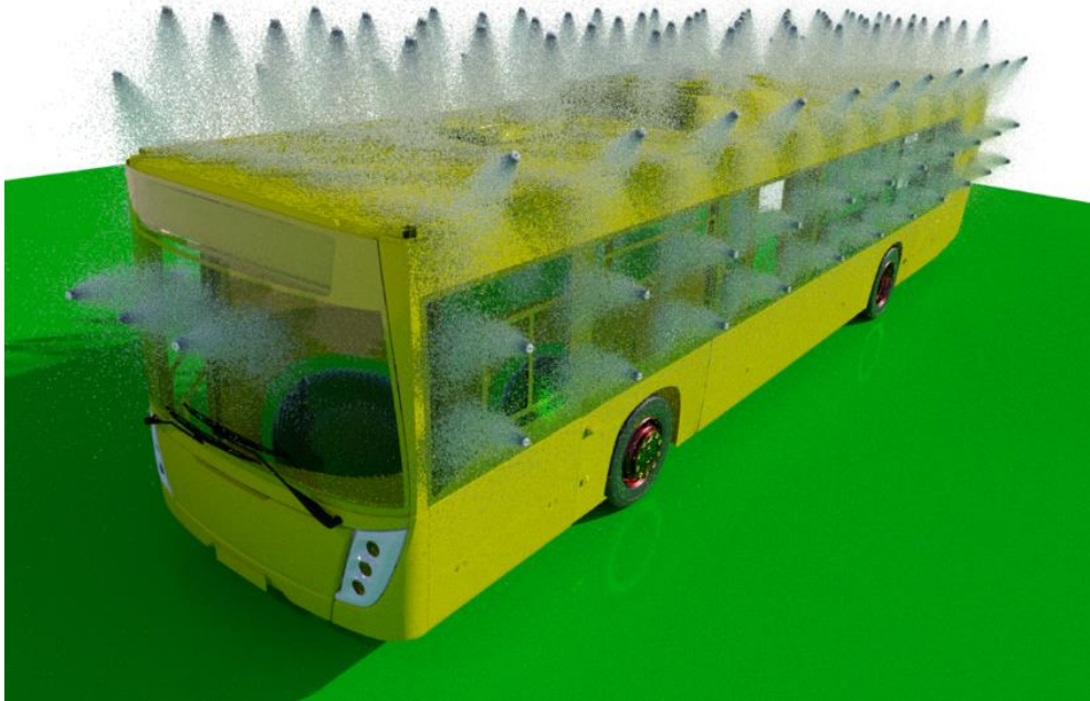
Fig. 6. Element of the graphical user interface of the virtual test bench for water protection and drainage of the vehicle body.
