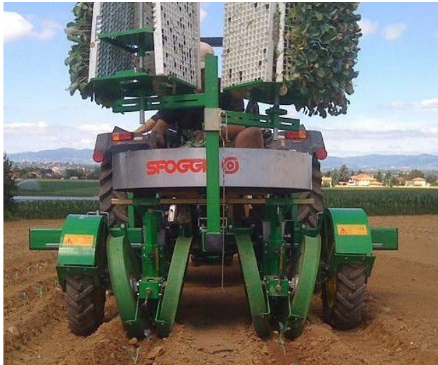
Fig. 2. F-18. Semi-automatic planting machine
