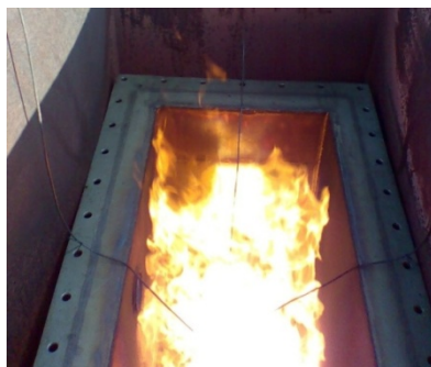
Fig. 5 Flame structure during the preliminary experiments on the 3 modules afterburner functioning on natural gas
