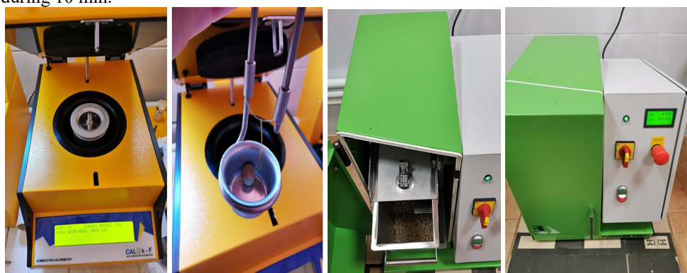
Fig. 3. Determination of calorific value and durability of feed pellets
