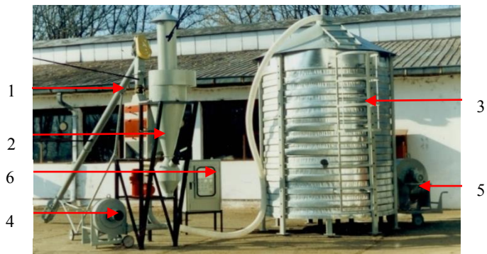
Fig. 1. Installation for storage and preservation of cereals ISC10
