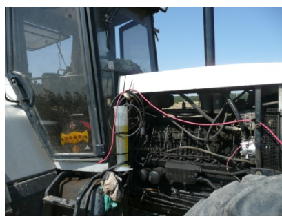
measuring the amount of fuel consumed during a test
