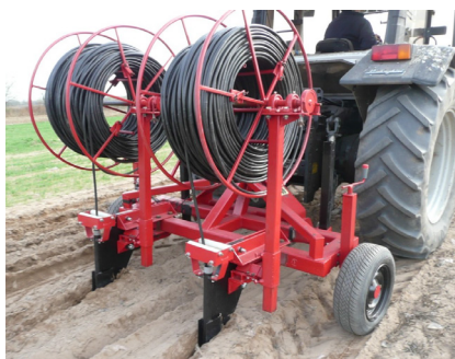
Fig. 1. The research object: equipment for burying drip irrigation lines in the ground
