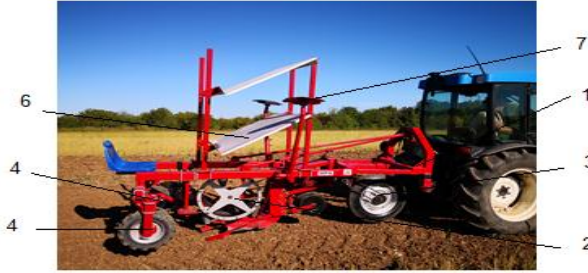
Fig.4 Machine for planting vegetable seedlings and herbs in a row, MPA symbol (**** INMA Bucharest, 2018) 1-Frame, 2- planter, 3- transmission, 4- rear support wheels, 5 –compaction wheels, 6- rack, 7- track marker
