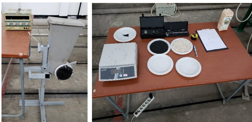
Fig. 8 Experimenting the electrically operated vegetable seed distributor
