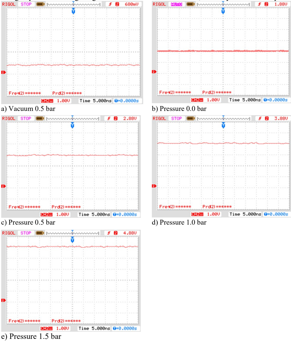
Fig. 8. Pressure sensor signals.
