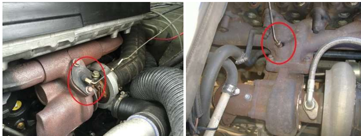
Fig. 5. Diagram of the system with the additionally placed sensors and experimental pictures.
