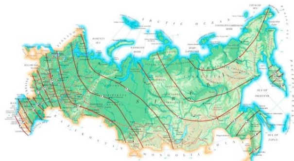
Fig. 2. Zoning of the Russian territory according to efficiency of topsoil thermal energy utilization in case of "horizontal" ground source system.
