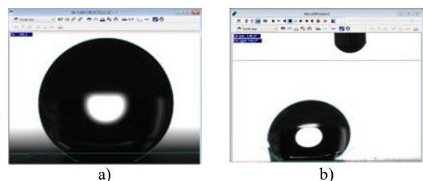
Fig. 7. Photo: OCA 20 device for measuring water contact angle and roll-off angle.
