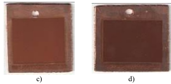
Fig. 6. Images of experimental samples with initial (a) and modified surface at laser fluence of 50 (b), 250 (c) и 900 (d) J/cm 2 .
