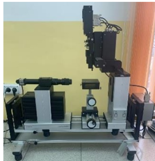
Fig. 7. Photo: OCA 20 device for measuring water contact angle and roll-off angle.
