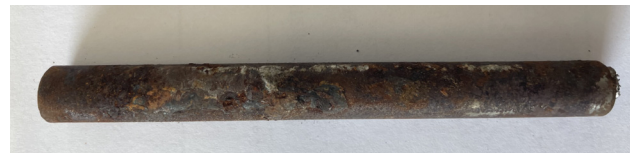
Fig. 12. The steel bar with 15mm protective layer in artificially fractured HYSZ after 40 S2D1 cycles
