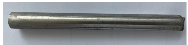
Fig. 14. The steel bar with 15mm protective layer in HYSZ after 40 S2D1 cycles
