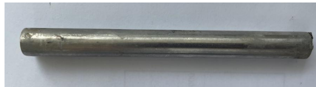
Fig. 13. The steel bar with 5mm protective layer in HYSZ after 40 S2D1 cycles
