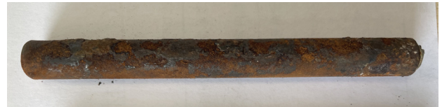
Fig. 11. The steel bar with 5mm protective layer in artificially fractured HYSZ after 40 S2D1 cycles
