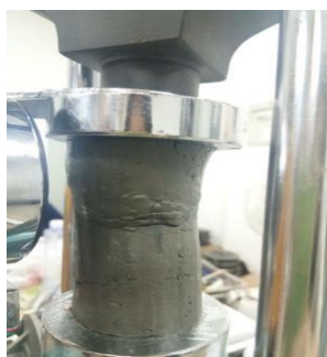
Fig.13. 25-2 Failure of undisturbed soil.
