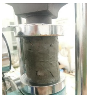
Fig.17. Damage of 2K-24 undisturbed soil.
