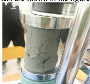
Fig.7. 14# Failure of undisturbed soil.
