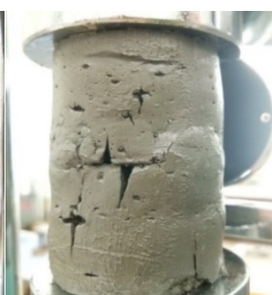
Fig.16. Remolded soil failure in Area B.
