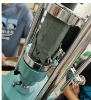
Fig.9. 21# Destruction of undisturbed soil.
