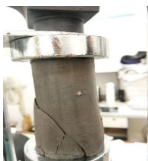
Fig.15. Failure of undisturbed soil in Area B.
