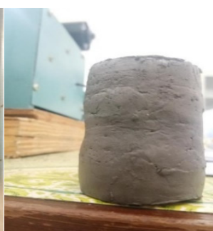
Fig.18. 2K-24 remolded soil damage.
