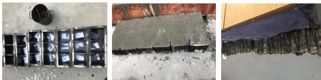
Figure 1. Concrete test mould, test block and impregnation method. (a) test mould; (b) test block; (c) Impregnation method.
