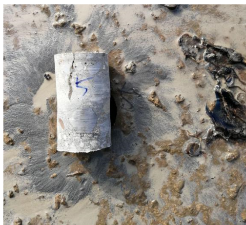
Figure 4. Diagram of the Crack Depth of No. 5 Hole
