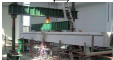
Figure 1. Schematic diagram of original beam reinforcement and test site diagram
