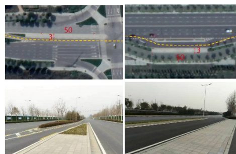
Figure 3. Island platform (left) and side platform (right).
