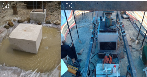
Fig. 8 In-situ direct shear test.
