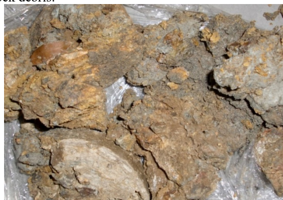
Fig. 2 The fault gouge of the F67 fault.
