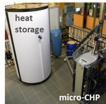
Fig. 7. Steam engine experimental set-up. [14]
