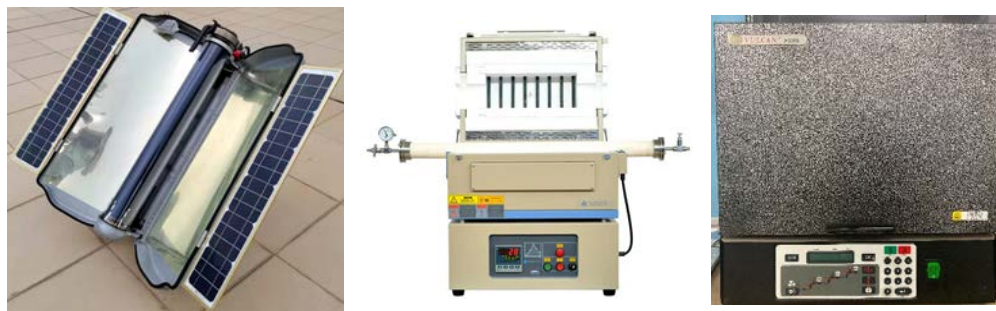
a. Solar pyrolysis device b. Tube furnace c. Muffle furnace
