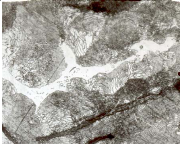
Fig. Large carbonitrides of titanium and vanadium in phosphide eutectic P = 0.30\% \times 800
